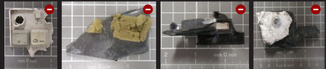
Polymer/polymer clipping, polymer/foam sticking, polymer/metal insertion, metal screwing [photos: Maris et al. 2015]
