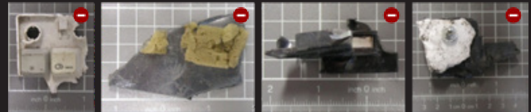
Polymer/Polymer clipping, polymer/foam sticking, polymer/metal insertion, metal screwing [Fotos: Maris et al. 2015]
