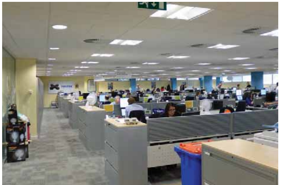
Figure 2.7 Open-plan office showing how furniture and general office life distracts from illumination on walls
