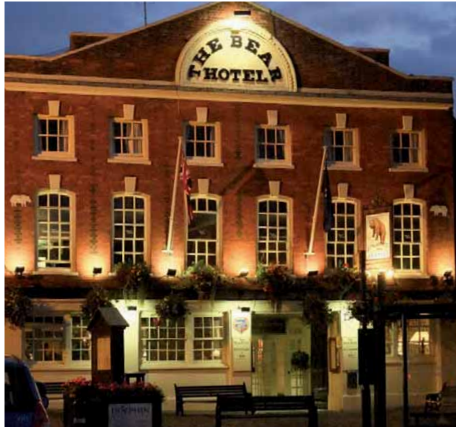
Figure 2.24 [above and right] Close offset floodlights mounted on a ledge
