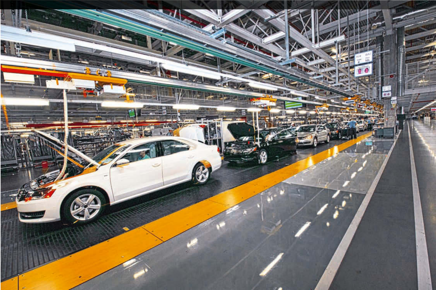
The Passat is manufactured for the American market on a very long production line.
